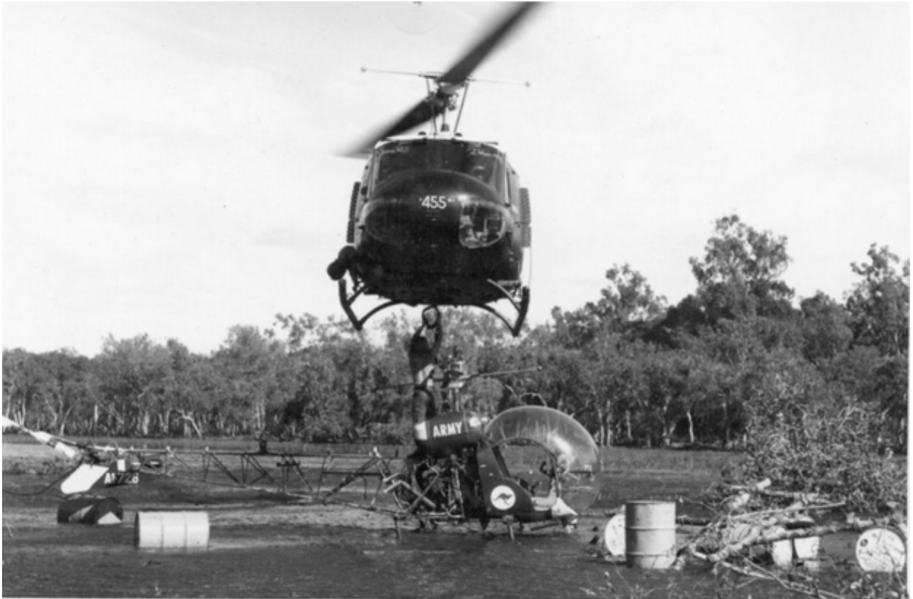
Bob Redman is standing on the Sioux ready to hook the rigging onto the Huey. The crewman, Monty Jesinowski can be seen leaning down from the left, guiding the pilot so that Bob Redman could slip the sling onto the external load hook of the Huey.
